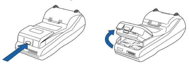
Figure 13 Removing the Smart Battery
